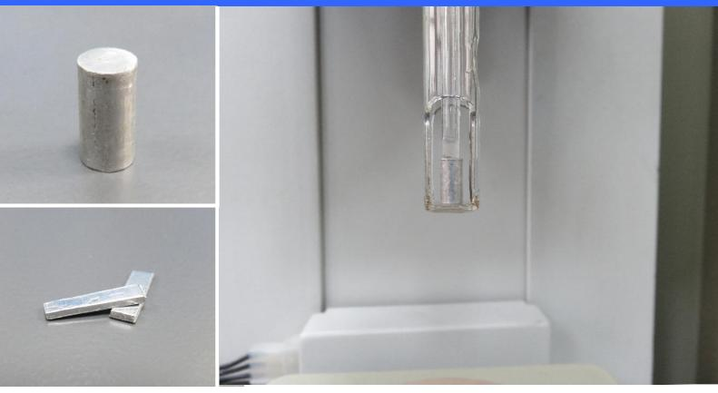
Ruston Services is able to provide high purity aluminium test pieces for thermal analysis expansion work. While this is not a traceable reference material, the high purity of the aluminium pieces ensures that the accuracy of the expansion measurements is high enough for most applications.
