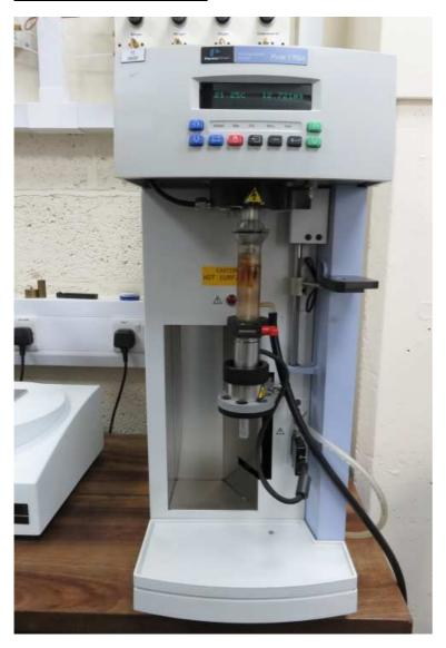
The vacuum hose supplied with the TGA Vacuum Control Unit should be connected directly to the TGA Pyrex furnace tube exhaust gas exit.
