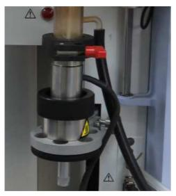
The picture (left) shows the vacuum hose connected to the purge exit on the TGA furnace protection tube.
